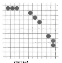
A dashed circular arc displayed with a dash span of 3 pixels and an *inter-dash spacing* of 2 pixels
