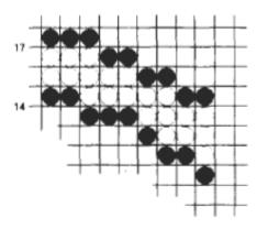
**Figure** 4.14 A circular arc of width 4 and radius 16 displayed by filling the region between two concentric arcs.
