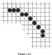
*Figure* 4.15 Circular arc displayed with rectangular pen.
